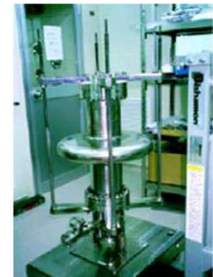
SC-cavity single cell test : 44 MV/m (2.1 K)
