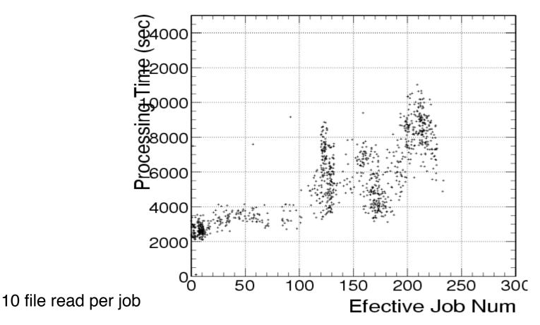
Apparent increase in spread of processing times per job for more than 100 simultaneous jobs.
