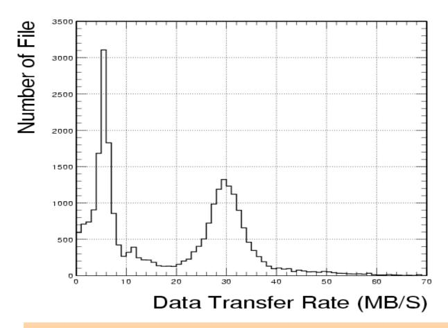
30 MB/s is a reasonable rate for transfering single file over the grid with 10 streams and average 10 file transfers a time Detailed structure not yet understood.
