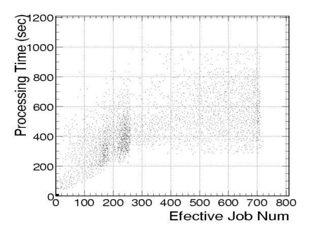
Average time per srmcp increases with # of simultaneous srmcp. Spread in time per srmcp increases with # of simultaneous srmcp.
