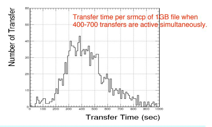
The scale test is characterized by many file transfer and each transfer only taking small amount of bandwidth, in contrast to loadtest, small number of transfer, each transfer taking a decent amount of network
