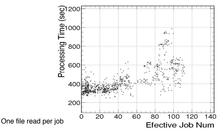
Apparent increase in spread of processing times per job for more than 70-80 simultaneous jobs.
