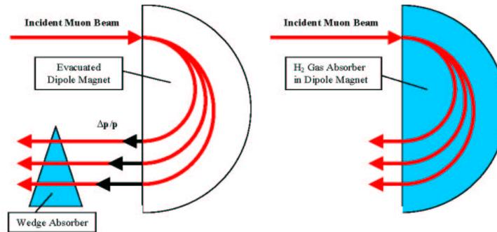
In a dipole, fast particles go at higher radius
