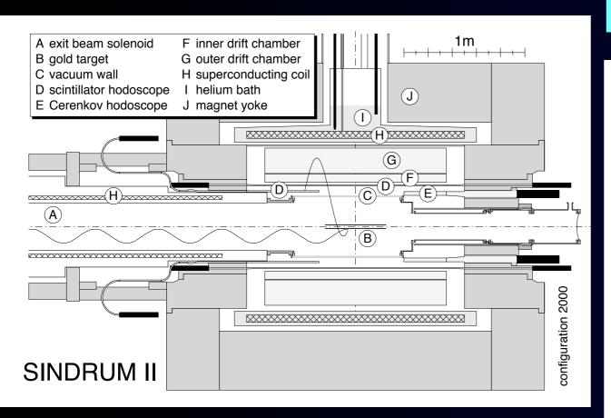
PSI muon beam intensity ~ 10<sup>7-8</sup>/sec beam from the PSI cyclotron. To eliminate beam related background from a beam, a beam veto counter was placed. But, it could not work at a high rate.
