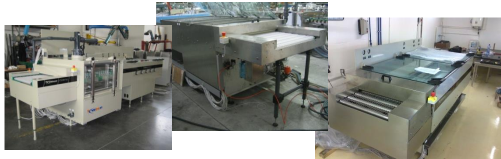
WISE Chemstar equipment: Industrial grade Cu and Kapton etch line for large GEMs
