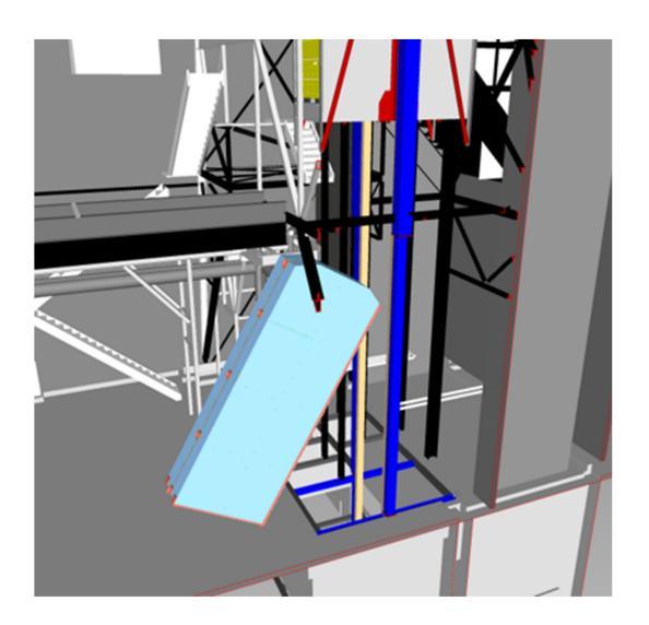
Guides for limiting rotation within shaft during lowering
