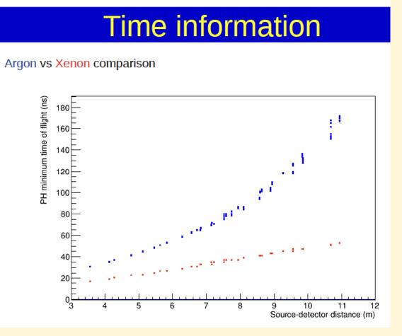
• FLUKA simulation for VD PD fallback Option (confirm MC results for  $4\pi$  PD
