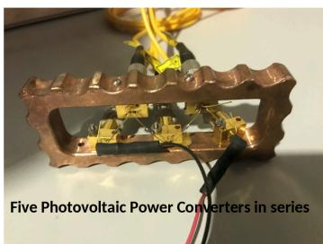
Tests PoF for supply bias V SiPM board in LAr (CERN 50 It test setup) [Nov-Dec.] - 60 V, 400 mA (Opto-Electric effic. 22% in cold)
