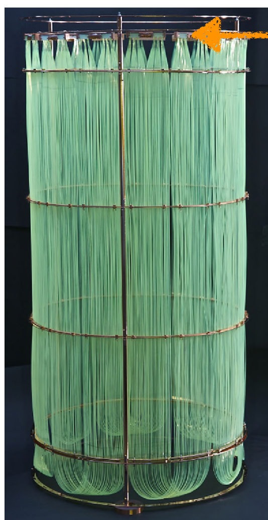
Fig. 14 The fiber curtain: height ~ 1 m, diameter ~ 0.5 m; 405 fibers read out on both ends by 90 SiPMs
