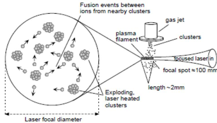
Figure 1 Layout of the deuterium cluster fusion experiment.
