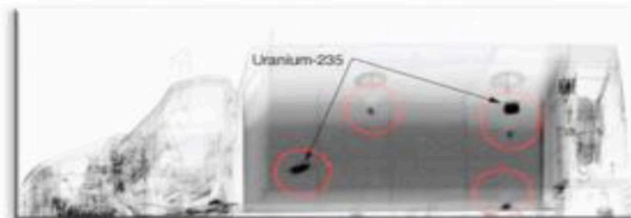
MEGAray beam absorption technologies currently under development could detect a piece of uranium-235 smaller than 5 millimeters in less than a second. This speed and accuracy would make the MEGAray system an excellent tool for examining cargo containers, trucks, and other loads on the move.
