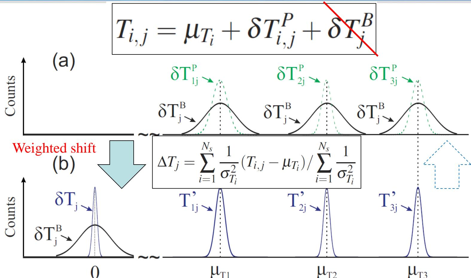
$$\sigma_{T_i}^2 = s_{T'_i}^2 + \frac{1}{\frac{1}{\sigma_{T_1}^2} + \frac{1}{\sigma_{T_2}^2} + \dots + \frac{1}{\sigma_{T_{N_s}}^2}}$$
