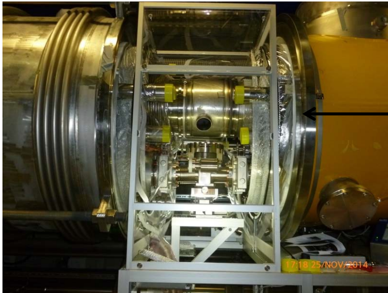
Portable clean room used at XFEL
