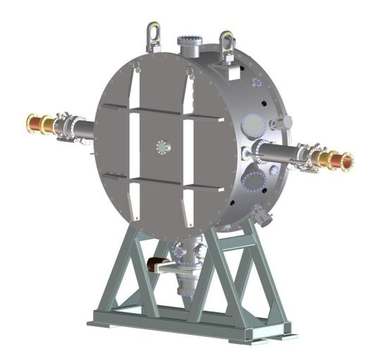
**RF** Module end plates are heavy, 3-400kg. Require hoist/frame in clean room. Cannot flow significant clean gas to preserve cleanliness because of fragile windows. **Replace Vac flanges with** thin/light 'clean' plates which allow insertion into beamline. Build structure around magnets and fit to clean room extension.
