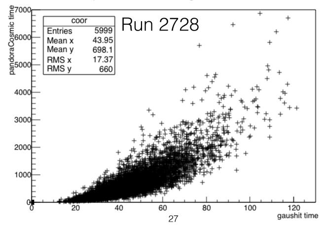
Chirping wires are the primary source of the excessive hit finding:
