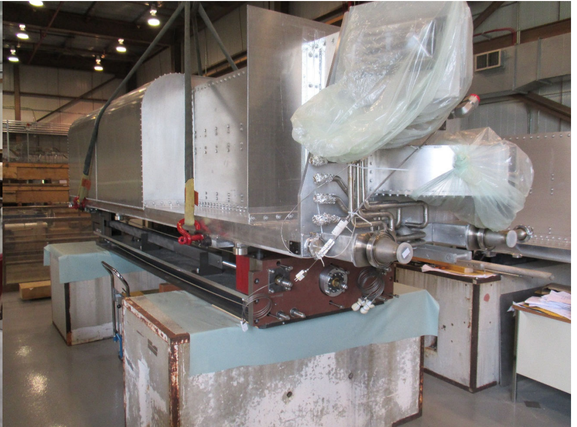
Checking for fit of Horn 3 to new adjuster module prior to installation.
