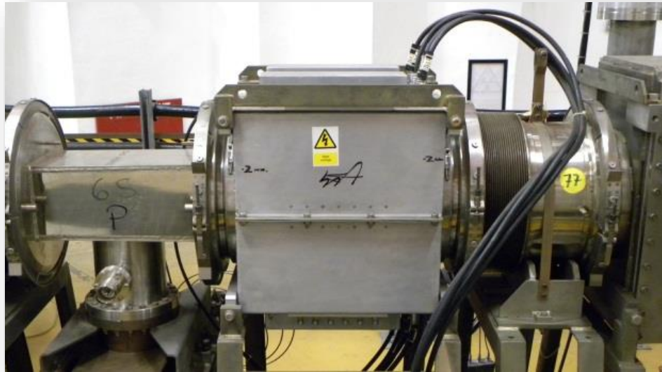
ISIS Vertical Betatron Exciter (Ferrite Loaded Kicker)
