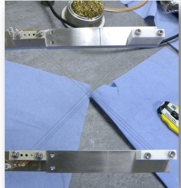
Detail of the wires on the bracket
