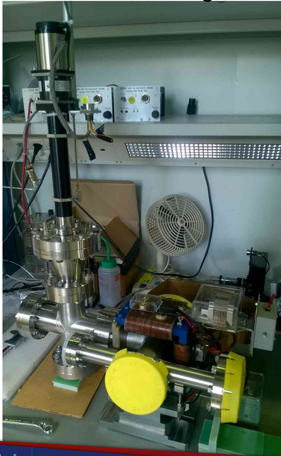
Diamond mover, and chamber with steerer magnet
