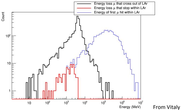
Three different sets of code give agreement on muon spectrum at 4850 ft to  $\sim 2\%$
