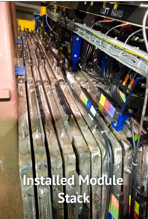
Modules have an outer detector frame of steel and scintillator...
