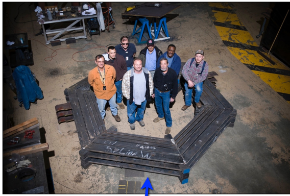
Modules have an outer detector frame of steel and scintillator...
