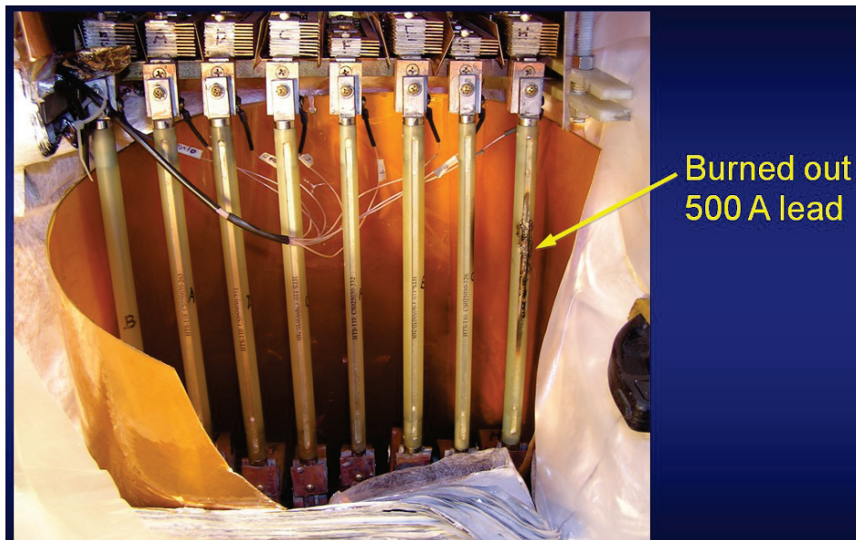
Fig. 1 Magnet 2 burned out HTS lead.
