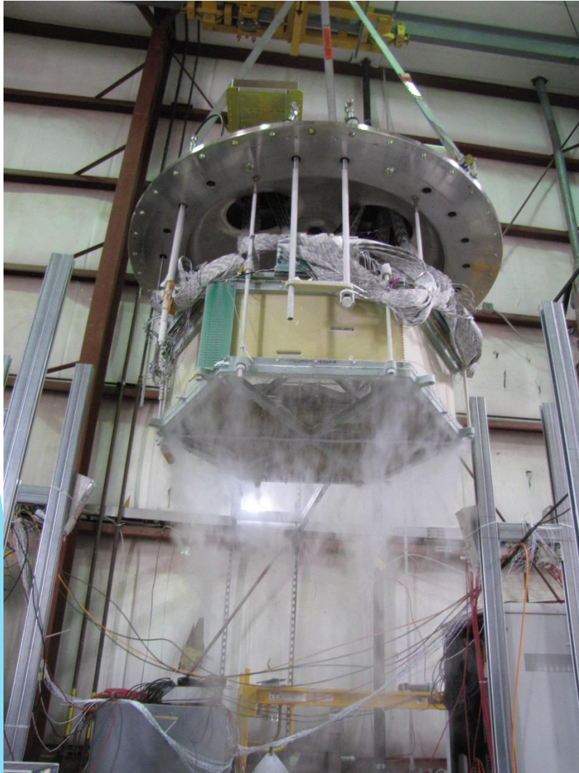
TPC being pulled out after liquid nitrogen run
