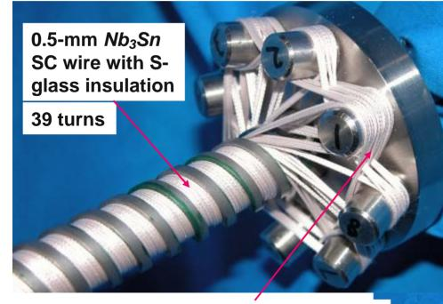
Undulator ends: designed for continuous winding of the double helix without any conductor joints and to minimize the stray field
