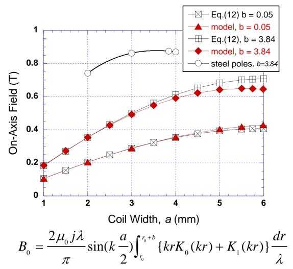
$\lambda = 12 \text{ mm}$  $r_0 = 3.15 \text{ mm}$
