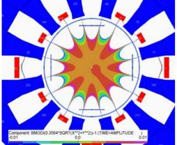
Field distortions because of eddy currents in BPM at 1 ms ramp, OPERA 2D TR.
