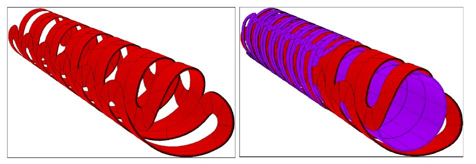
Helical Dipole modeled using current subelements in OPERA3D. MODIFY operations for current elements will help a lot in such cases.
