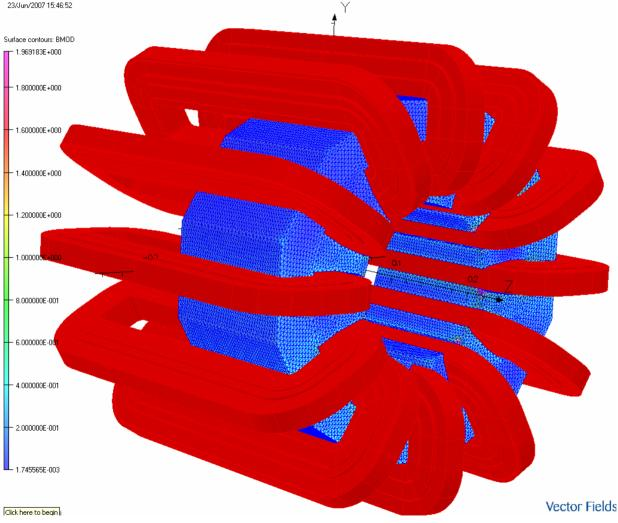
TOSCA code 4.2 million elements Shown variant when all coils powered by maximum current To check iron
