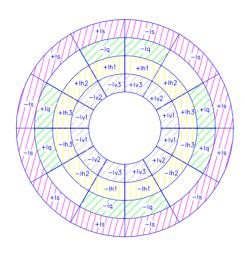
Dipole+Quadrupole+Sextupole Coil Currents:
