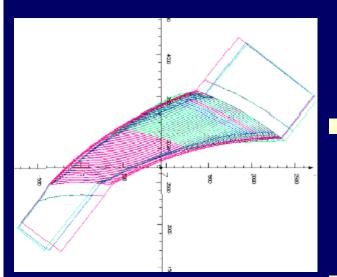
Effective length is measured at different radii on both sides of the magnet centre
