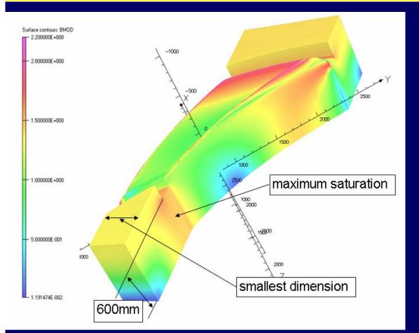
Maximum saturation imposes a very thick base plate (600mm)
