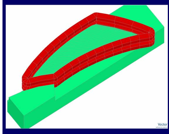
Enlarged the base plate to reduce thickness (480mm)
