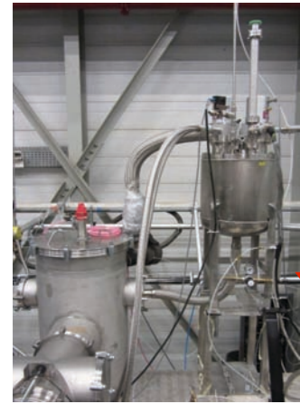
closed system: condenser (500 W cryocoolers)
