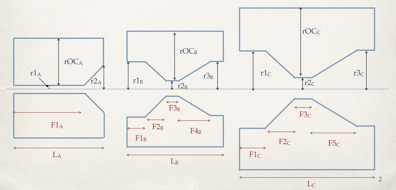
Horn lengths are defined sligtly differently than I've done in the past. I'm going to set one total horn length, then each segment's length will be a variable fraction of the total length. This will make it mechanically easier to study the dependence of results on total horn length (rather than individual segment length)
