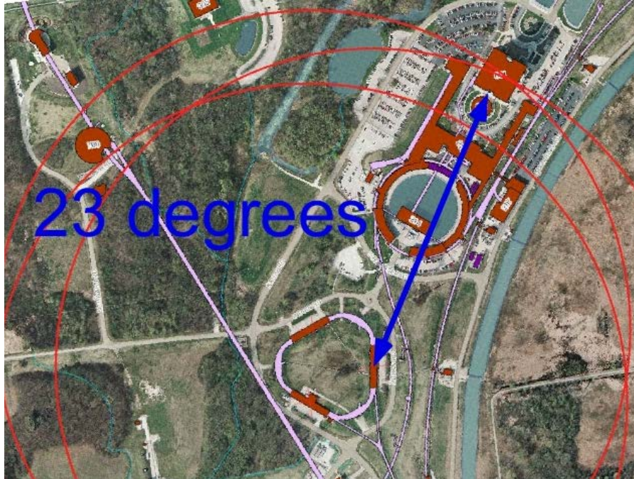
Figure 10 The red circles have a radius of 500 m; each one is centered at one of the service building footprints. The azimuthal angle between the z axis of the MARS simulation (parallel with the major axis of the AP30 service building) and the center of Wilson Hall is indicated by the blue line.
