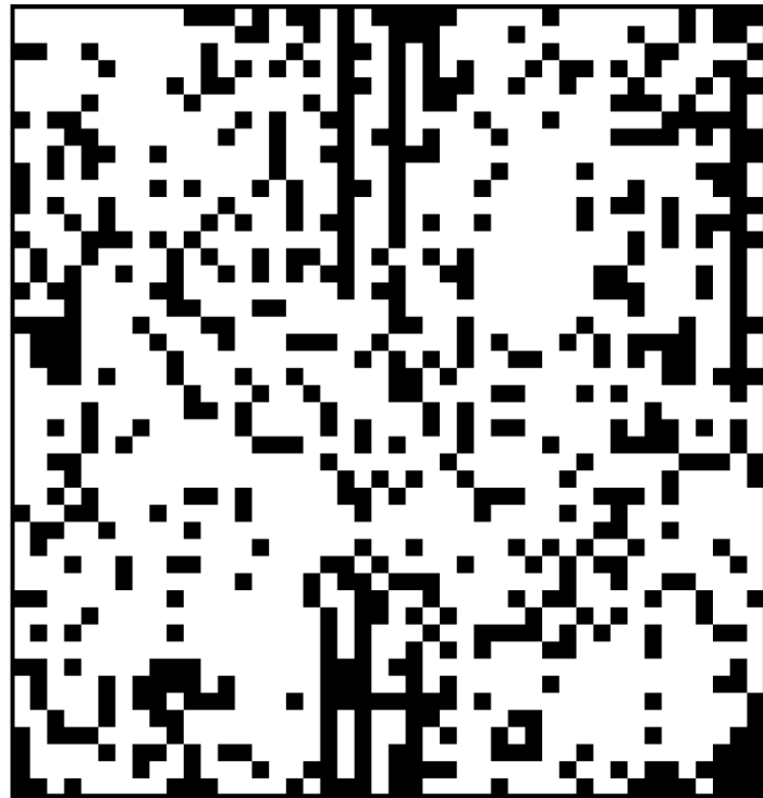
Figure 10. The results of beam mapping the ARCONS array. Pixels with good locations are shown in white. Vignetting is apparent at the bottom right side of the array. The overall pixel yield in this engineering-grade array is \sim 70\% .
