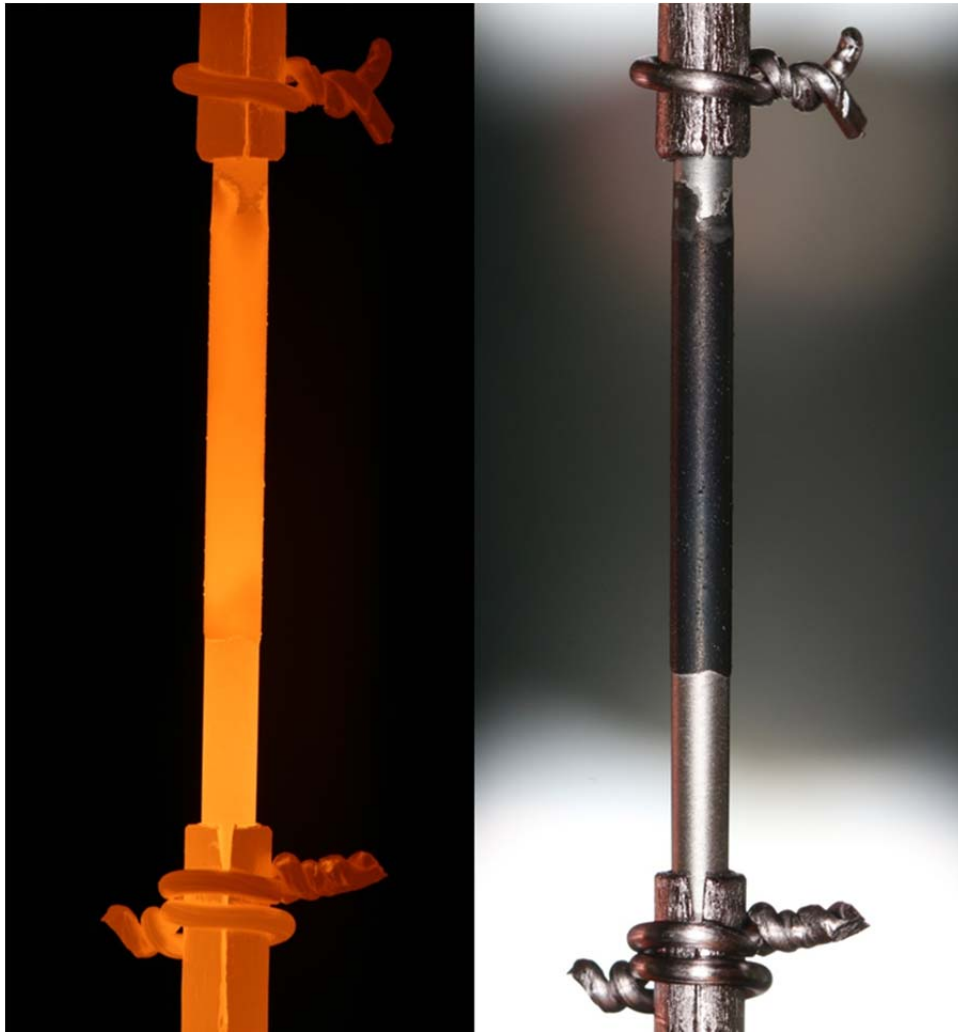
Figure 36, The sample after 40 days bake-out at 1250°C, hot (left) and at room temperature (right).
