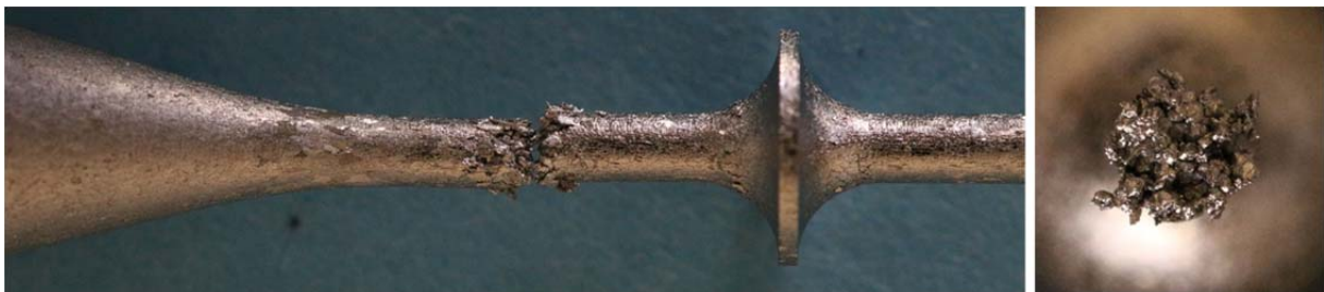
Figure 8, Close up view of the failed sample (left) and an end view of the failure surface (right).
