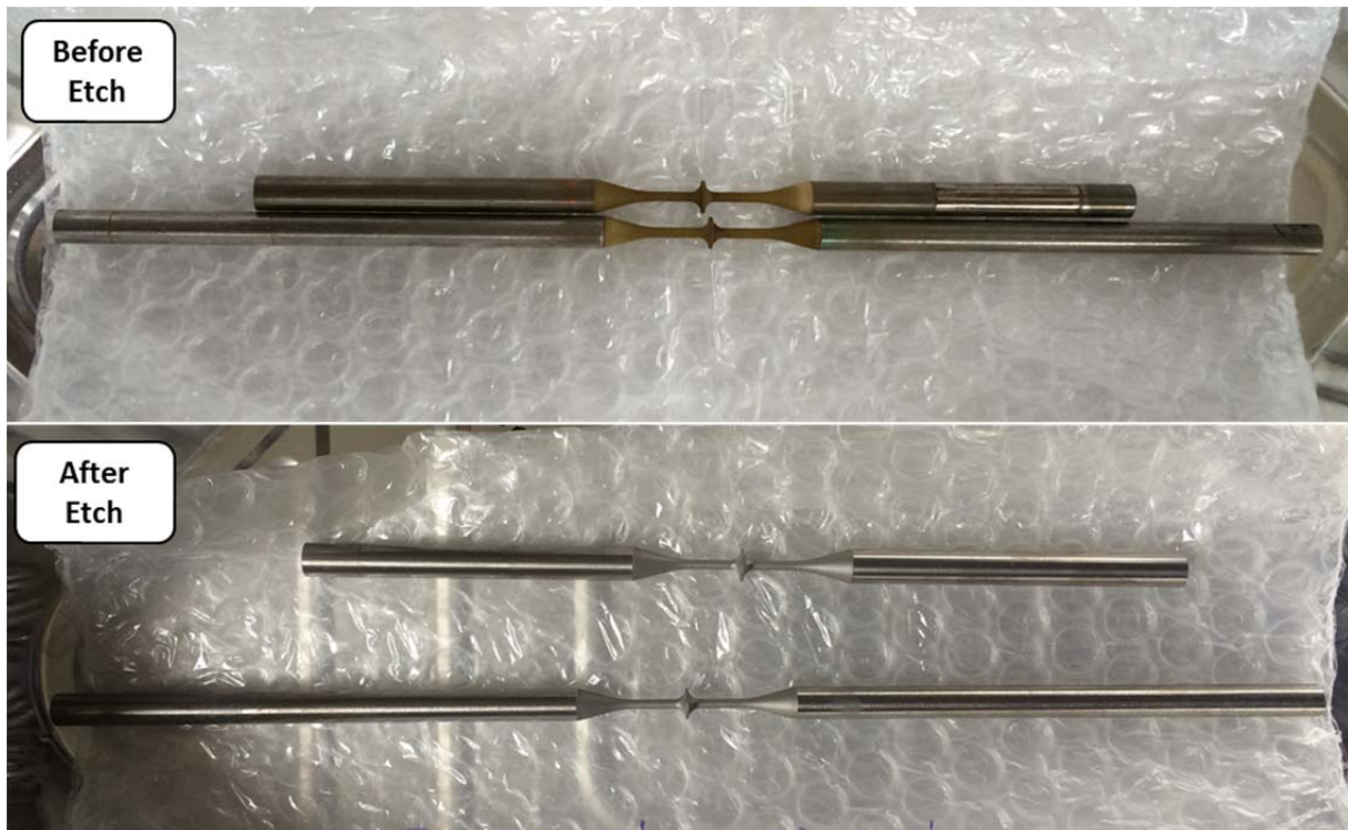
Figure 10, “Long” and “short” samples before (top) and after (bottom) etching.
