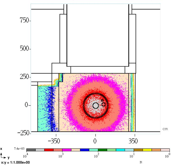
Cross section, 4 feet from extraction tube flange
