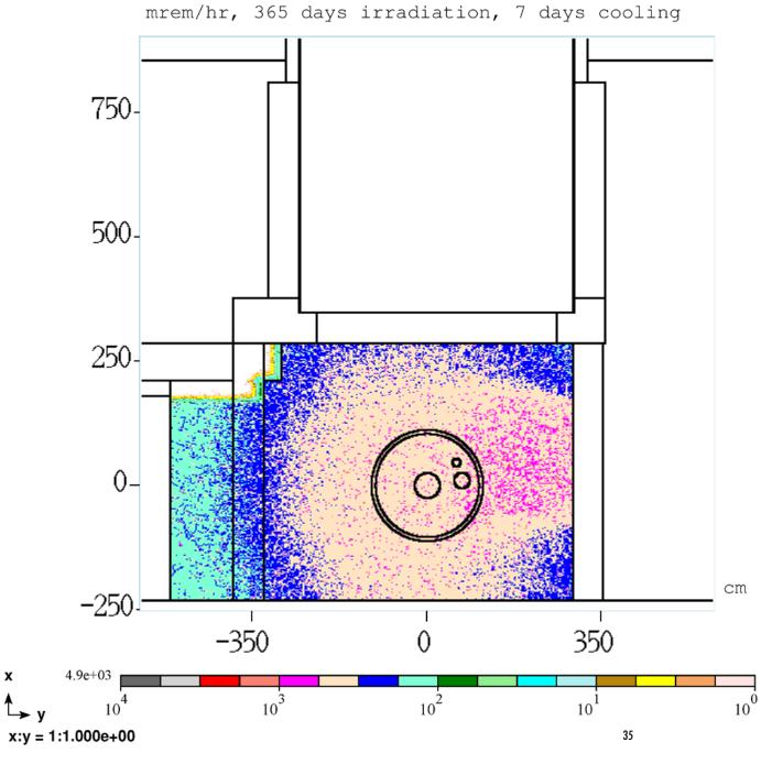
Cross section, 18 feet from extraction tube flange
