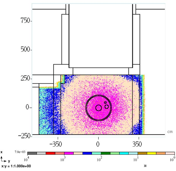
Cross section, 13 feet from extraction tube flange
