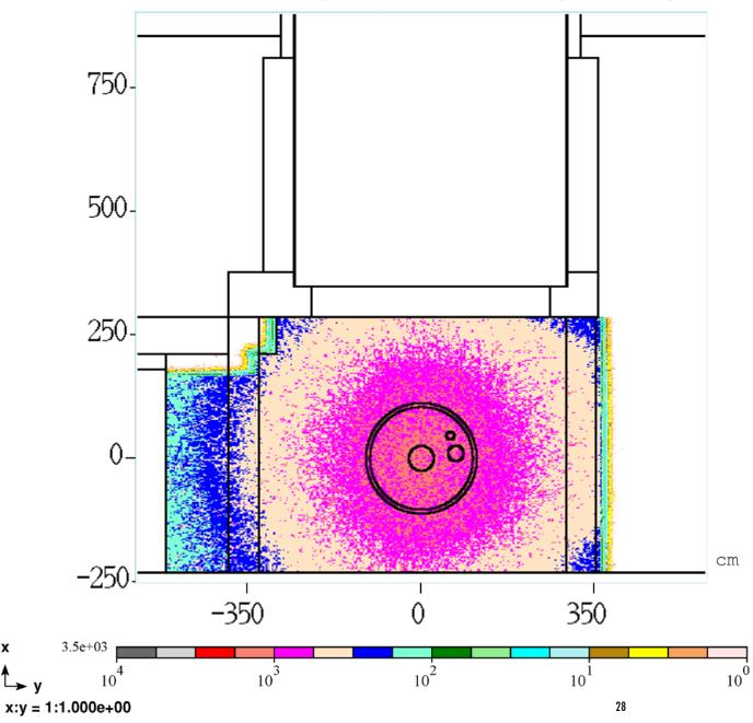
Cross section, 11 feet from extraction tube flange
