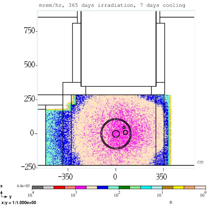
Cross section, 14 feet from extraction tube flange
