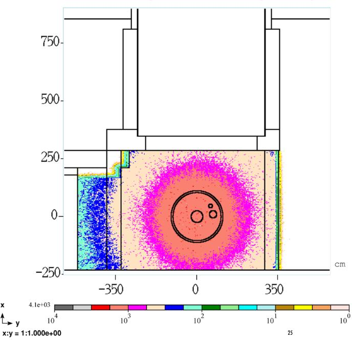
Cross section, 8 feet from extraction tube flange
