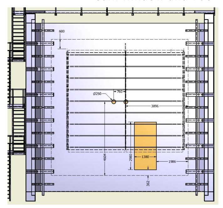
The vertical placement of the TPC needs to be set soon as this affects where the beam will enter the drift volumes. Current distance is 600 mm from membrane to top of electronics fin.
