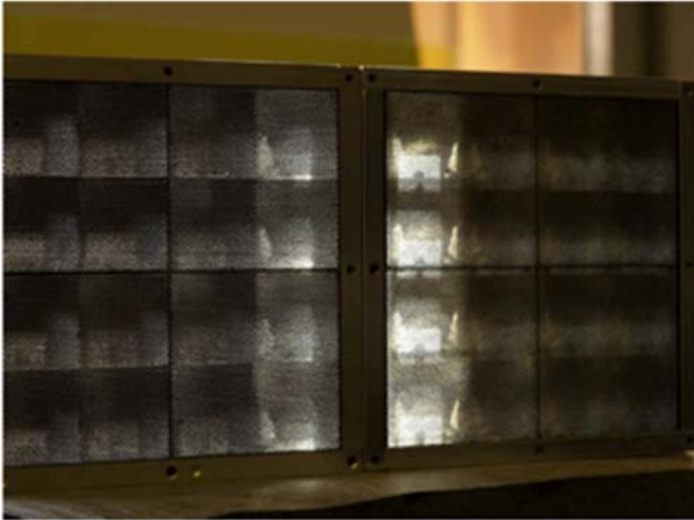
Figure 1: Two EMCAL prototypes from the side opposite to readout. The new EMCAL prototype has much finer sampling frequency compared to the old prototype.
