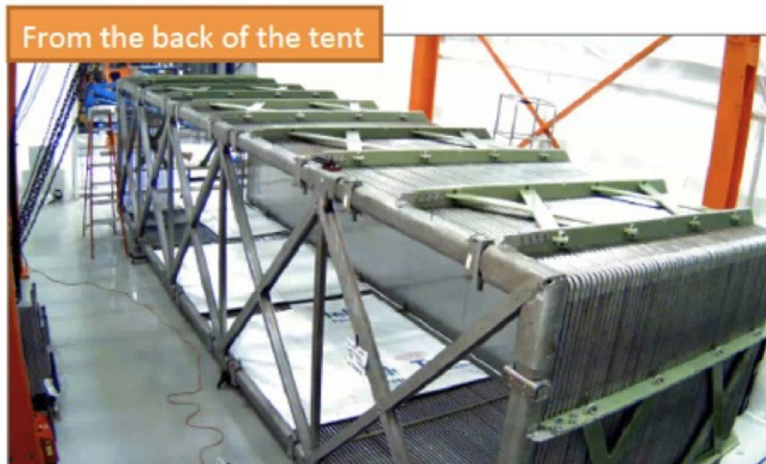
Figure 2: Photograph of the MicroBooNE TPC as it was being assembled at the DZero Assembly Building before being inserted in the cryostat and transported to LArTF.
