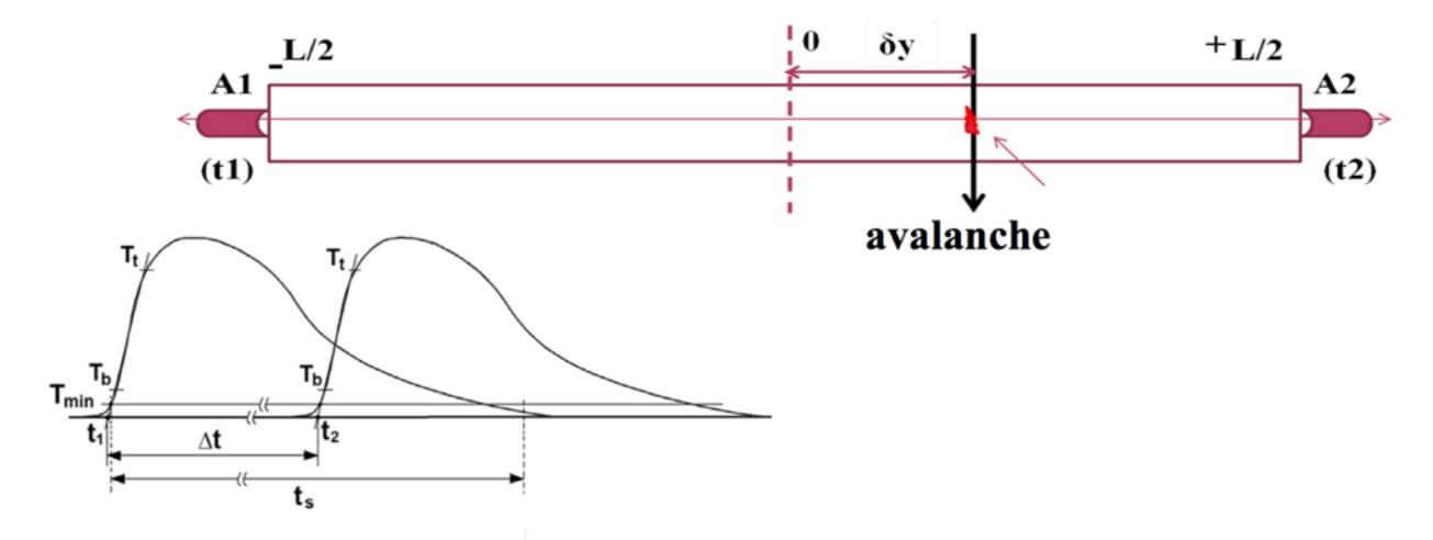
The point of the avalanche is  $\delta y$  from anode center. Signals arriving at amplifiers pass the distance  $L/2 \pm \delta y$ , where L is the anode length. So,  $\Delta t = 2\delta y/v$ , where v is the signal propagation velocity along the anode wire, and the direction from the straw center is determined by the sign. The v = 3.49 ns/m. 1 cm distance corresponds to the difference in the time delay = 69.8 ps.
