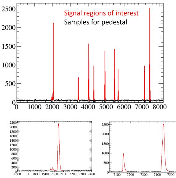
1<sup>st</sup> step to find region of interest and pedestal for a given channel In addition some FFT noise filtering can also be performed
