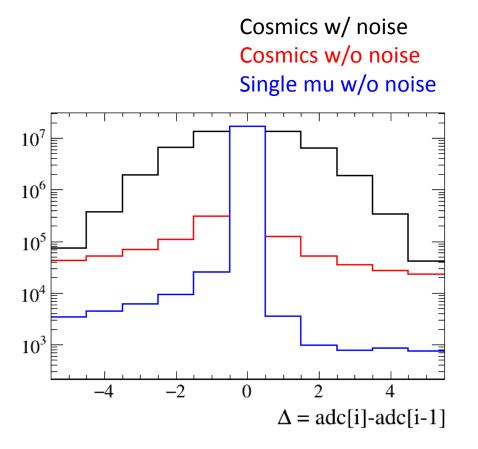
Huffman coding scheme to encode  $\Delta(ADC_i - ADC_{i-1})$  same as in uBooNE
