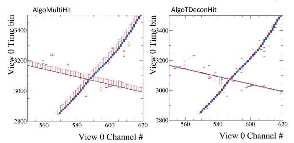
Split ROI into several regions if several peaks are detected. Integrate waveform in each region to find charge. ← simple & fast : suitable for online processing Deconvolve true charge distribution from response using least-squares fit  $\leftarrow$  slow (good for specialized offline studies e.g., diffusion) 7
