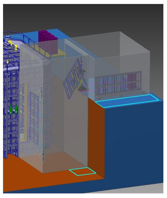
The actual clean space enclosure needs to be designed and supported. Most probably a tent like structure similar to what was used in MicroBoone.
