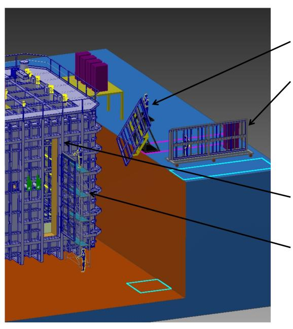
Rotation fixture for APAs and potentially CPAs with access platform.
