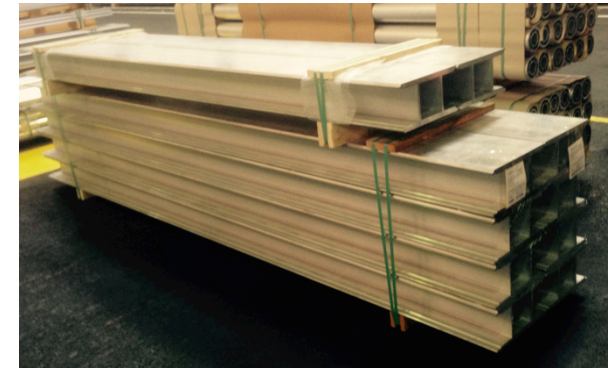
U-frames extruded profiles
