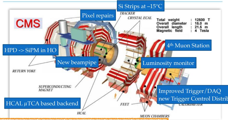
Coming into the start of Run2, CMS was a ~new detector Ready on 3 June 2015 for first collisions at √s=13 TeV
