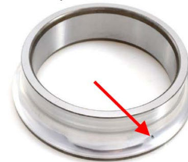
Fig. 2: The inner ring with 2 flaked areas. One flaked area is identified by the arrow.
