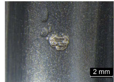
Fig. 3: Detail photo of the flaked area from Fig. 2.
