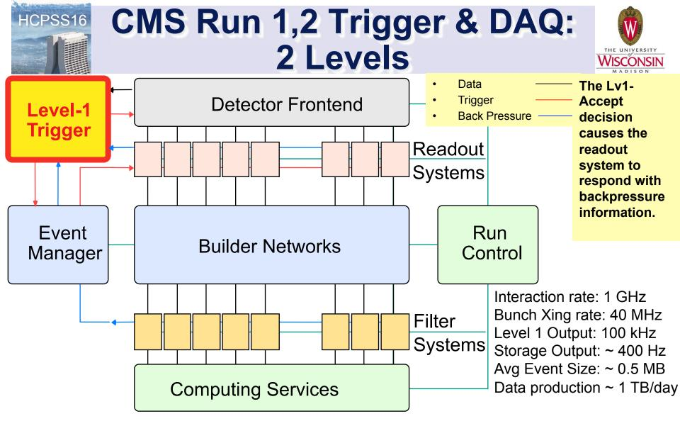
Lv1 decision is distributed to front-ends & readout via TTC system (red). Readout buffers designed to accommodate Poisson fluctuations from 100 kHz Lv1 trigger rate.
