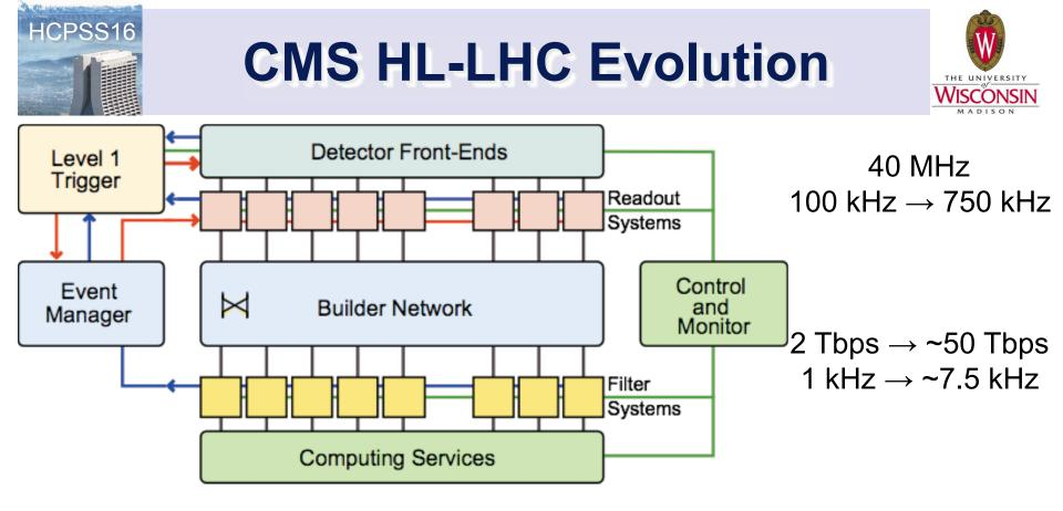
HL- LHC: Lumi = 5 - 7 x  $10^{34}$ <PU> = 140 - 200 (increase × 6 - 8 v. run 1) E = 13-14 TeV (increase ~ 2 v. run 1) 25 nsec bunch spacing (reduce × 2 v. run 1) Integrated Luminosity > 250 fb<sup>-1</sup> per year
