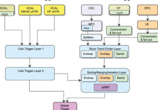
Generate L1A and send via TCDS distribution to detector front-ends to initiate readout Maximum round-trip latency 4 µs Data stored in on-detector pipelines
