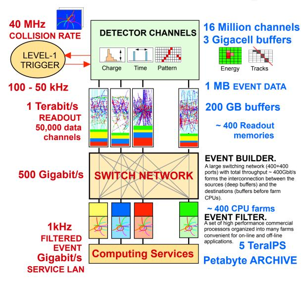
**Challenges:** 1 GHz of Input Interactions Beam-crossing every 25 ns with ~ 23 interactions produces over 1 MB of data
