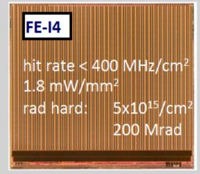
130 nm technology pixel size 250 × 50 μm<sup>2</sup> 70 M transistors
