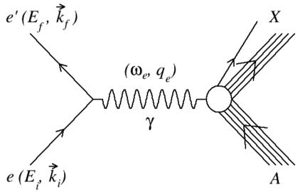
$$\left(\frac{d^2\sigma}{d\omega_e d\Omega}\right)_e = \frac{\alpha^2}{Q^4} \left(\frac{2}{2J_i + 1}\right) \frac{1}{k_f E_i} \times \zeta^2(Z', E_f, q_e) \left[\sum_{i=1}^{\infty} \sigma_{L,e}^J + \sum_{i=1}^{\infty} \sigma_{T,e}^J\right]$$
