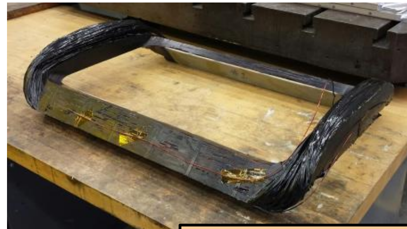
Quadrupole coil with controlled end build and total length
