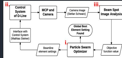
iii. Image analysis of beam spot after MCP/Camera
