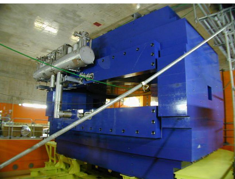
Coils with cryostats, LHe vessels
