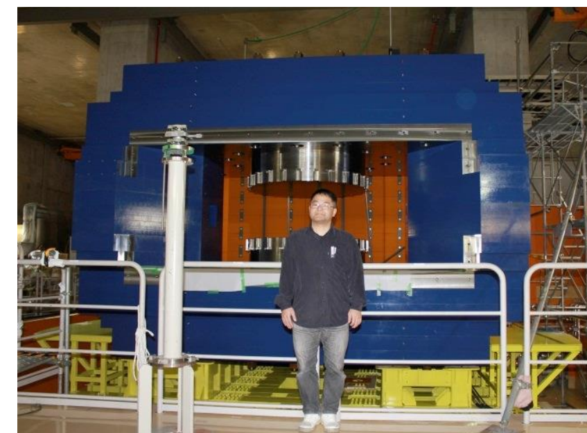
Magnet yoke with poles
