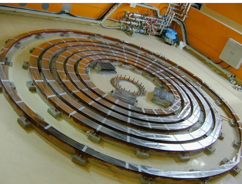
Rails for rotatable base
