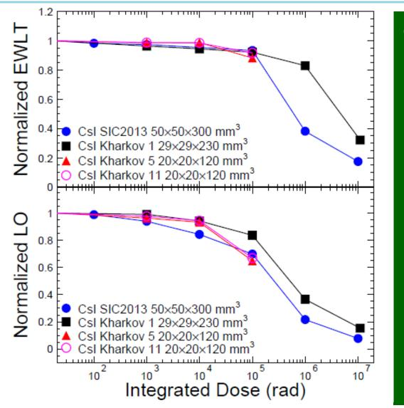
Consistent radiation hardness: no significant degradation in LO and LRU up to 100 krad, but not beyond.
