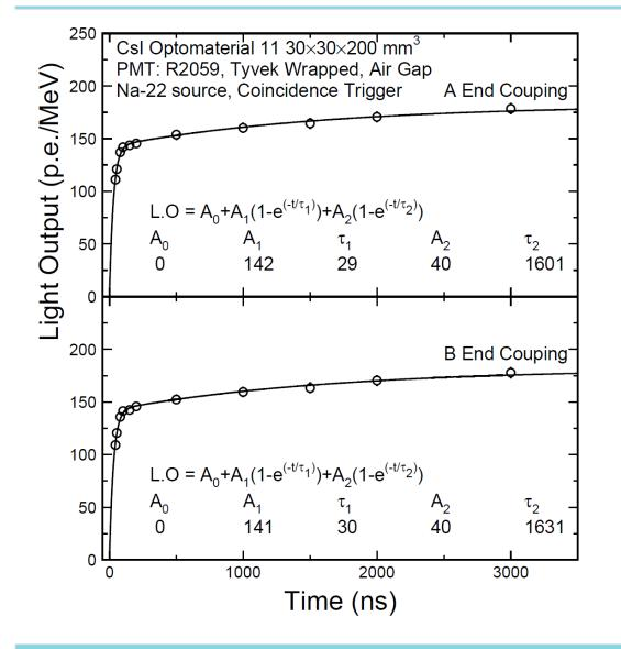
A position independent slow component with a decay time of 1.6 us was observed, which is at a level of 30% of the fast component
