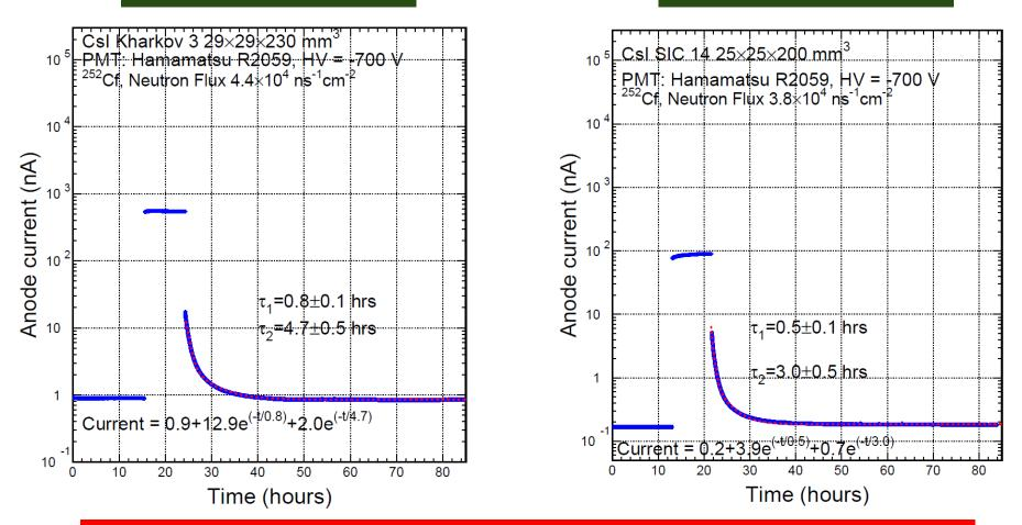
Neutron induced photo-current is much less than that from gamma-rays
