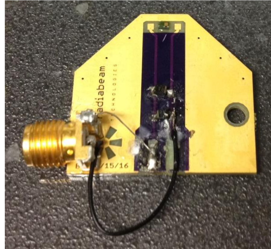
RadiaBeam PCB for PCA chip. Top-side (left) and bottom-side (right)
