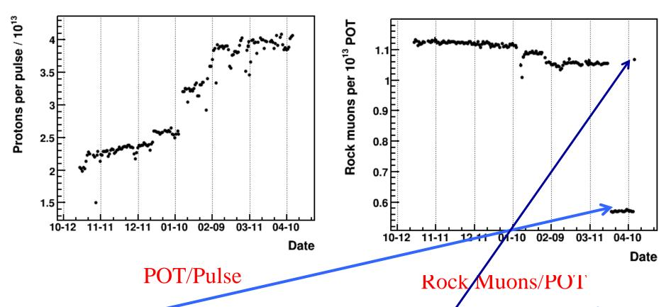
• The problem with the rock muon plot due swapping of chain 1-2-3 to 1-6-3 on Mar 25 is fixed. The rock muon rate is back to its nominal rate.
