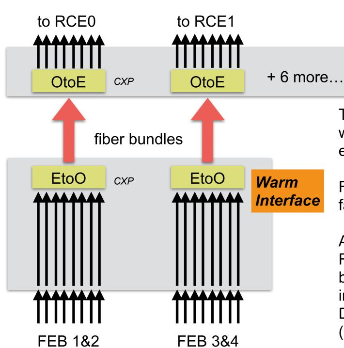
This follow the spirit of 35ton, where the RCE FPGA is the first "smart" element to see the data...
