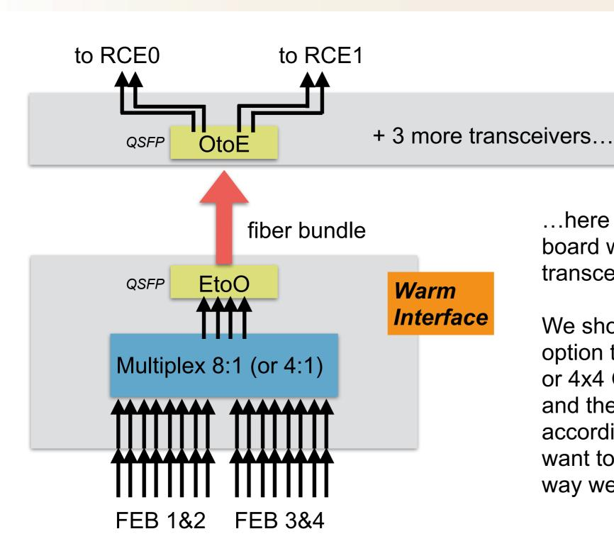
...here is the SNBD-like warm board with a single QSFP transceiver.
