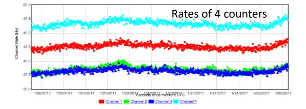
After correcting for barometric pressure, students can also study dependences on other variables (temperature).
