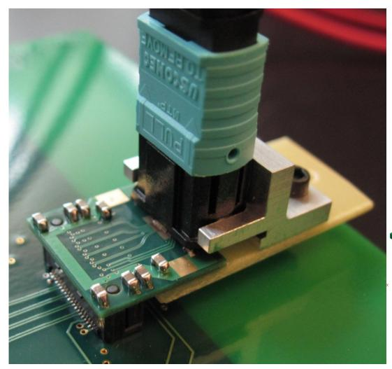
Connector secured to optoboard with screws instead of
